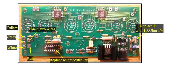
3) Gently pry the old microcontroller from the socket, and insert the new PIC16F688.
